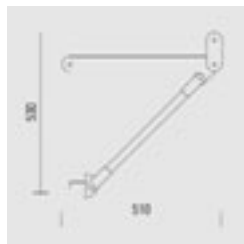
second arm with strut for double pole
